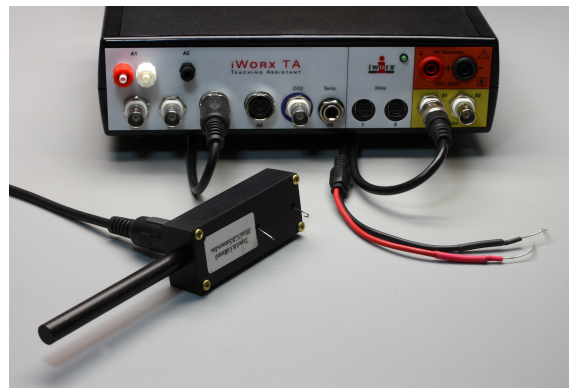
Figure 2: The C-BNC-N2 stimulating electrodes (left) and FT-302 force transducer (right) with the CBNC- N2 stimulating electrodes connected to the IXTA.
