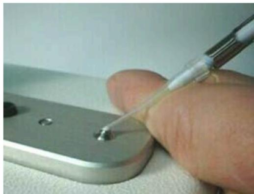
2. Close the sampling arm. The sample column is automatically drawn between the upper and lower measurement pedestals. Click the “Blank” button (F3)
