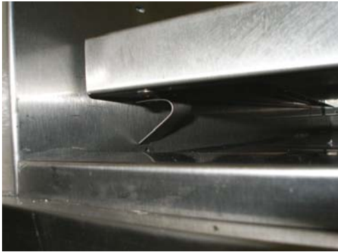
Photo 11: Detail of the Bottom Shelf support
