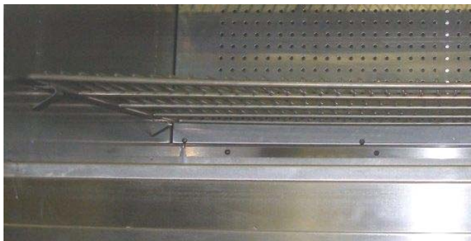
Photo 49: Bottom wire shelf. Notice the position with respect to the back wall plenum
