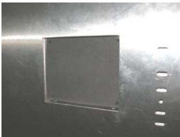
Photo 19: Small insulation covering the fan compartment
