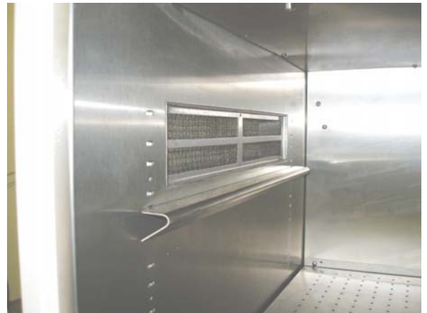
Photo 13: Air filter installed in its compartment. Again, notice the position of the lamp canopy support with respect to the filter
