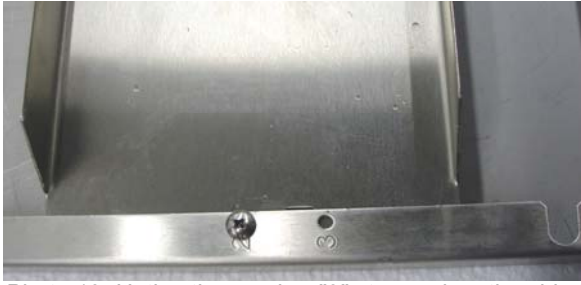
Photo 13: Notice the number "2" stamped on the side flange
