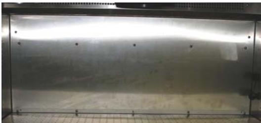
Photo 19: 5 screws installed at the Back plenum before installing the top shelf
