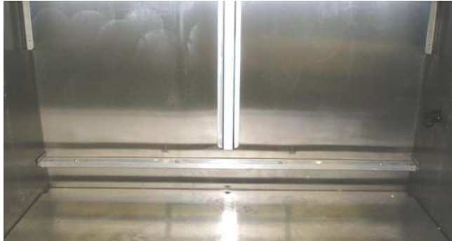
Photo 10: A1000 view after Installing the Back Plenum Bottom Panel
