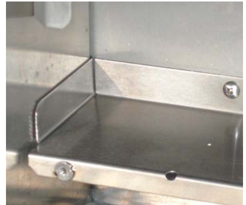
Photo 2: A1000 view after Installing the Back Plenum Bottom Panel
