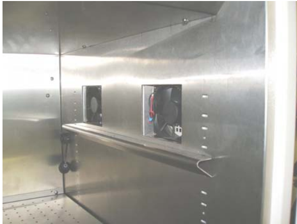
Photo 12: Fans Installed and plugged in to their compartments. Notice the position of the lamp canopy support with respect to the fans
