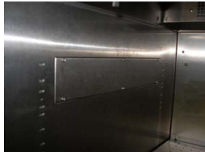
Photo 33: Air inlet cover installed
