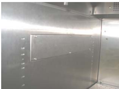
Photo 46: Air inlet cover installed
