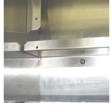
Photo 40: A1000 view after Installing the Back Plenum Bottom Panel
