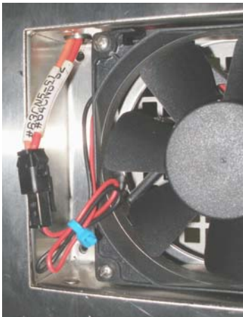
Photo 8: The fan wire connector has a single orientation connection – ensure the connections 'snaps' together.
