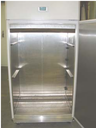
Photo 47: Canopy support showed with 18" (450 mm) between them for maximum growth height
