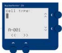
3. The cursor blinks at the starting position. Scroll through the character set by using the “Up” and “Down” button (3,4) to enter the desired text and move to the consecutive character positions with the functional button “>>” (6). By using the functional button “<<” (5) the cursor moves one step back and deletes the entered character.
