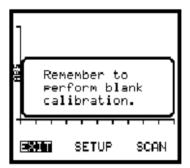
Select **SETUP** and adjust the wavelength value as appropriate for the test being performed.
