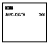
When the required wavelength value has been entered and confirmed, place a sample blank into the sample chamber and close the lid. Press **CAL** and the instrument will perform a calibration as shown.
