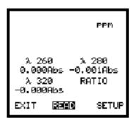
The DNA calculation will be performed by reading the absorbances at the required wavelengths and calculating the answer based on the pre-entered factors.
