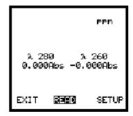
Remove the sample blank from the chamber and insert the unknown sample. Close the sample chamber lid. Select **READ** and the instrument will measure at both points (even when only 280nm is required):
