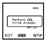
Place a sample blank into the sample chamber and close the lid. Press CAL and the instrument will calibrate at 260/280nm or 260/230nm, depending on the mode selected.
