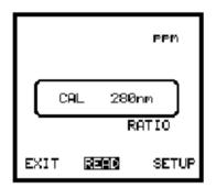
If the reference wavelength option is selected a third calibration will be performed at the nominal reference wavelength of 320nm. All 3 values will be shown on the instrument display.
