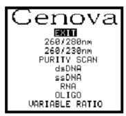
Set up and measurement procedures are the same for 260/280nm and 260/230nm modes, as detailed below. Select the appropriate mode of operation: 260/280nm or 260/230nm and the following screen will be displayed:
