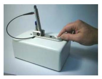
4. Analyze an aliquot of the blanking solution as though it were a sample. This is done using the "Measure" button (F1). The result should be a spectrum with a relatively flat baseline. Wipe the blank from both measurement and pedestal surfaces and repeat the process until the spectrum is flat.
